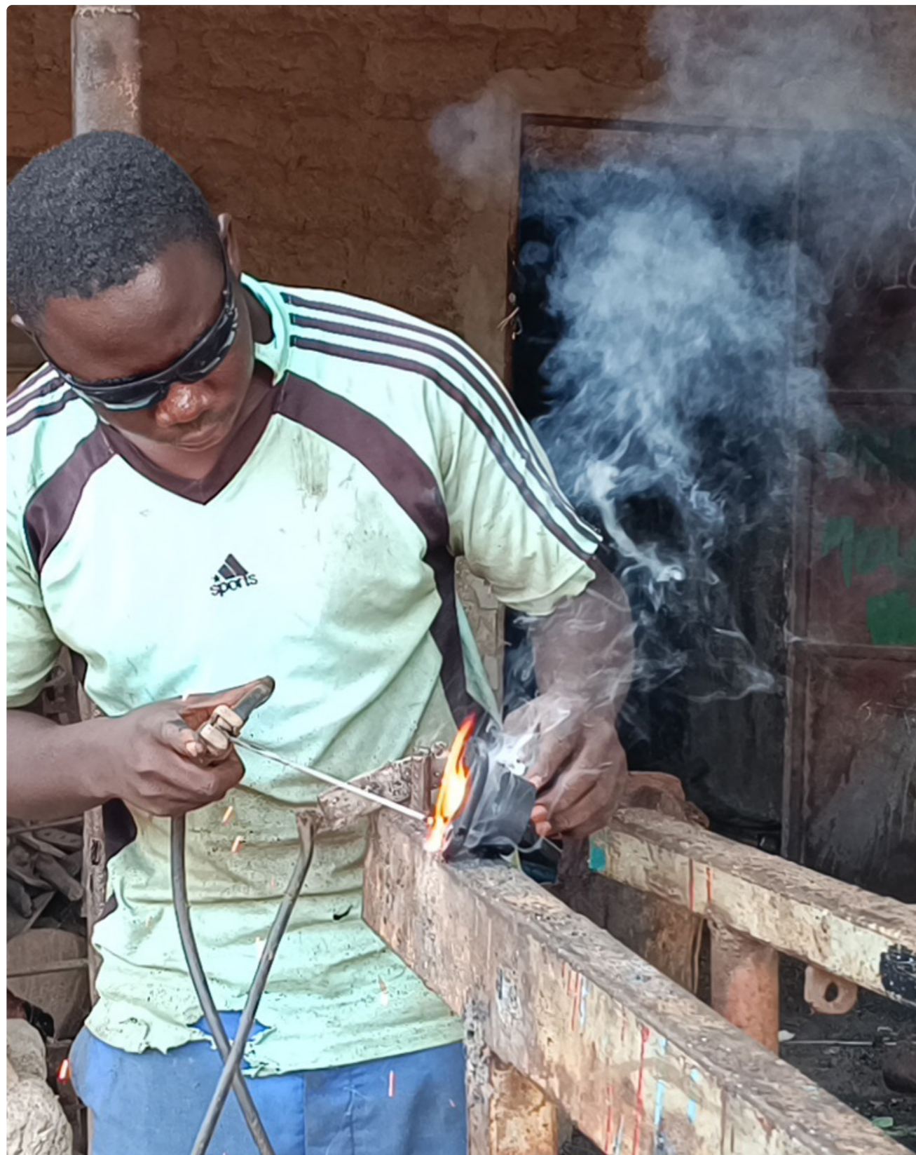
Belem Souleymane repairing a motorcycle part in his welding workshop UNCDF / Touré Monia Roxane
