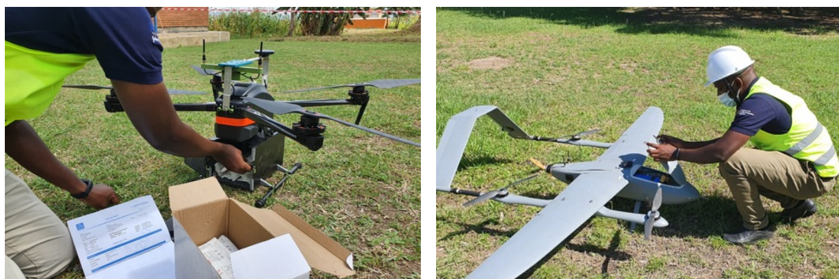
Figure 3.6: Flight testing Multi-rotor drone with cargo box (L) Fixed wing drone being loaded with COVID-19 swabs (R)
