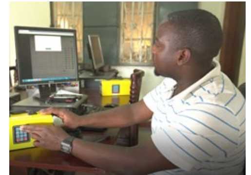
Edmund Osama, Head of IT at Eco Group, demonstrates how to turn on the solar kit using a code generated from the Eco Pre-Pay dashboard.
